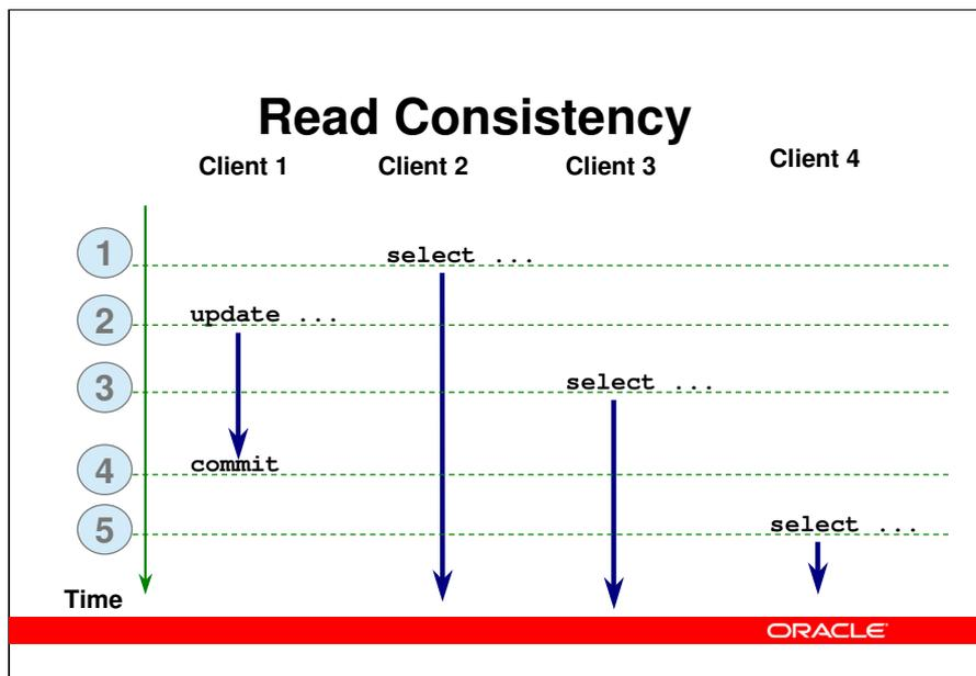
The behaviour of the *read consistency* model is described further in this slide:
