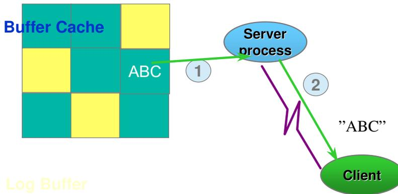
1. The buffer cache contains exact copies of blocks on disk, where data is stored in the block format shown previously, with typically several rows per block.
