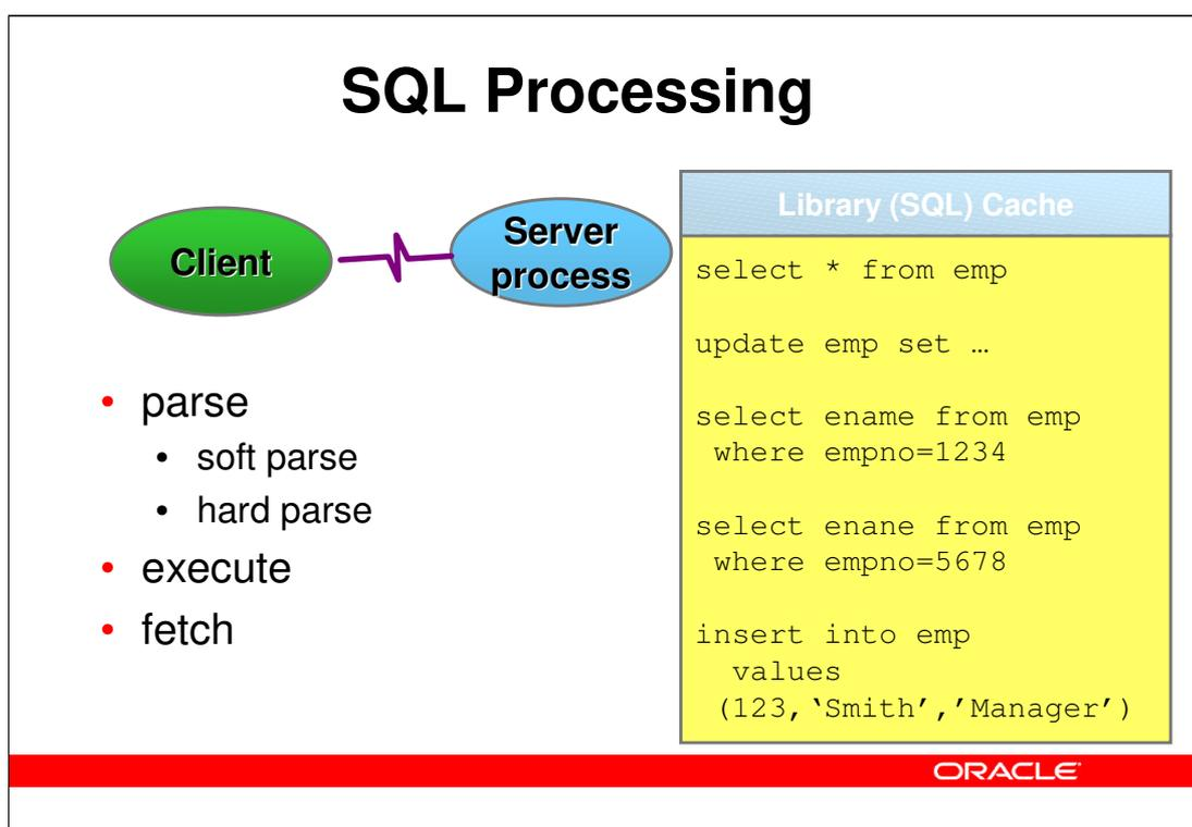
Oracle SQL processing is done in generally three steps via the client/server interface; SQL statements are sent to the server, are being executed at the server and results are sent back to the client. For optimization, the number of roundtrips between the server and the client should be limited, as each roundtrip incurs a network message or a process switch if the client and the server runs on the same computer.
