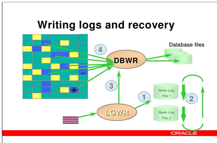
This slide shows some details of the way the log writer and the database writer work together. In general, there are at least two redo log files, and the set of files are used sequentially; when one fills up, the next log buffer is written to the next redo log file.
