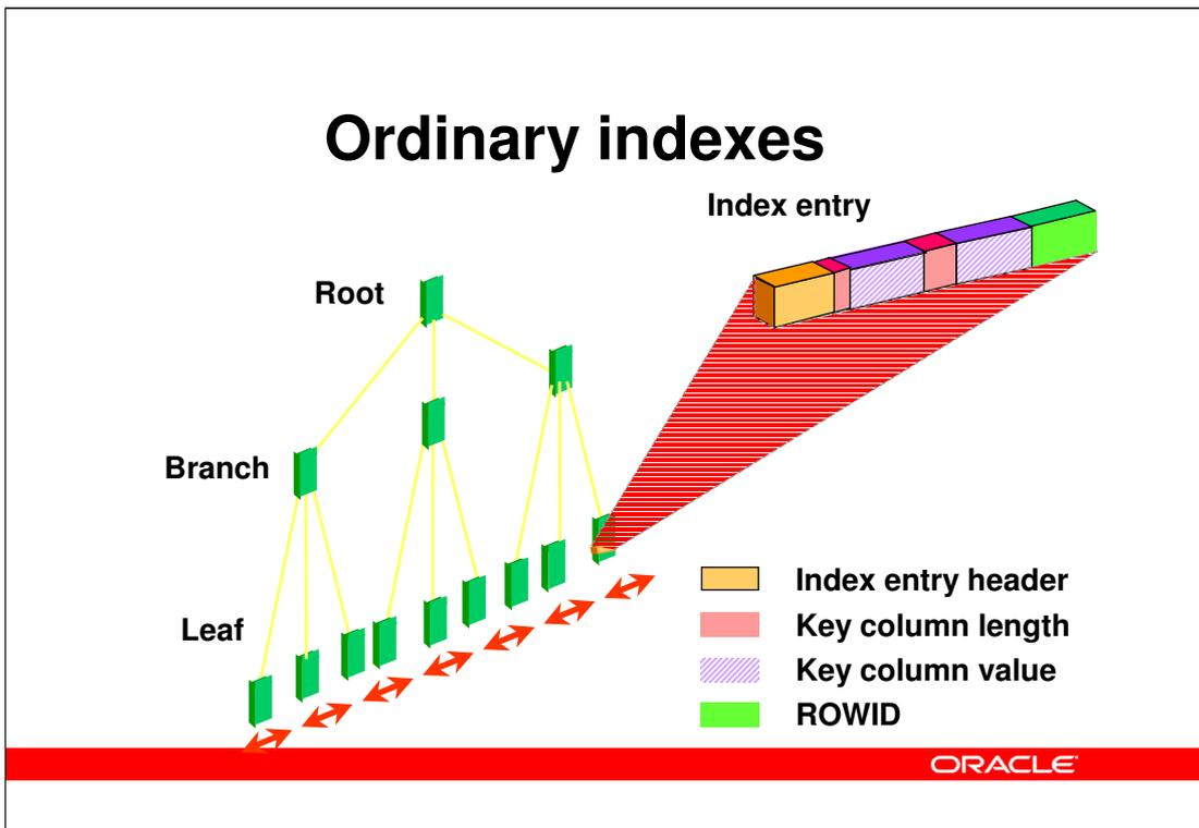
Ordinary indexes are binary and contain one or more levels of branch blocks (the top one being the root), and one level of leaf blocks. Each index entry stores a header, the actual column values and a rowid pointing at the data block. In case of an index organized table, the rowid part is replaced by the full row of the table.
