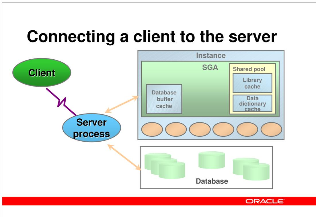
The client process runs in its own address space (actually as its own operating system process, quite often on a separate computer), completely separated from the Oracle Instance by the network or the inter process communication. Hence, the client cannot attach to the SGA, and cannot read or write to the database files.
