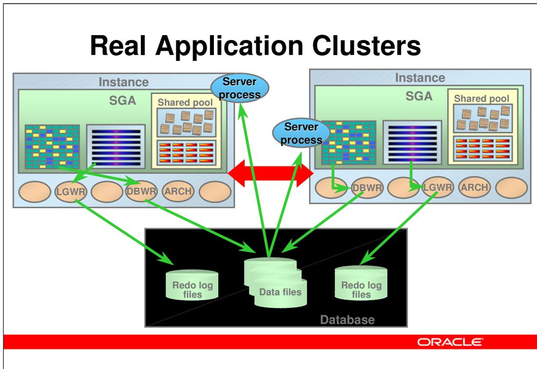
In Real Application Clusters, there are multiple instances (normally one per database server node) serving a single database. The single database is stored on a set of disks, that are *shared* between all instances.
