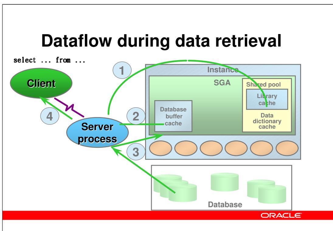
During queries (SQL select statements) data is found in the actual database, i.e. in the database files, and the server process, that is connected to the client together with the other parts of the Oracle instance is responsible for executing the SQL statement, getting data from the database and sending these to the client.
