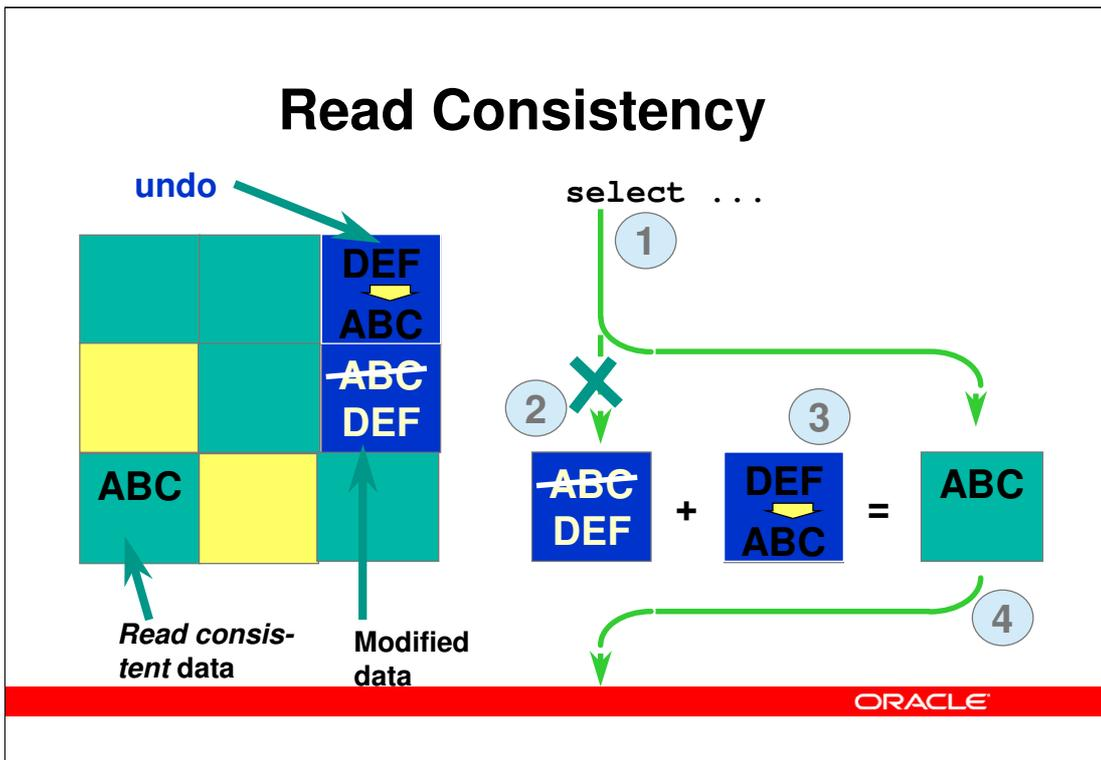
The undo (rollback) information, that was discussed on the previous slide, is used in other cases, besides an actual rollback operation from the client. In the scenario above, some user has updated the block with “ABC” into “DEF”, which is actually changed in the data block and registered in the undo block as rollback information. Concurrently, some other user is performing a query.
