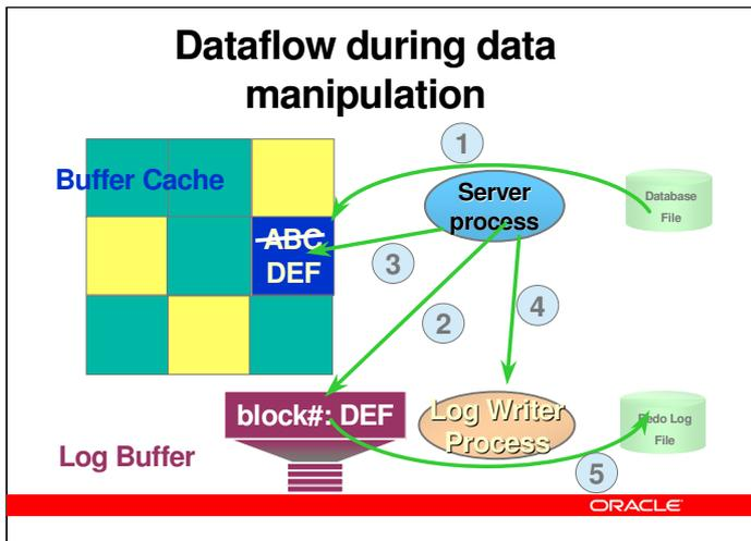
During processing of a data manipulation statement (DML, i.e. SQL insert, update or delete), the basic processing is like for queries. I.e. handling of SQL and the library cache is the same.
