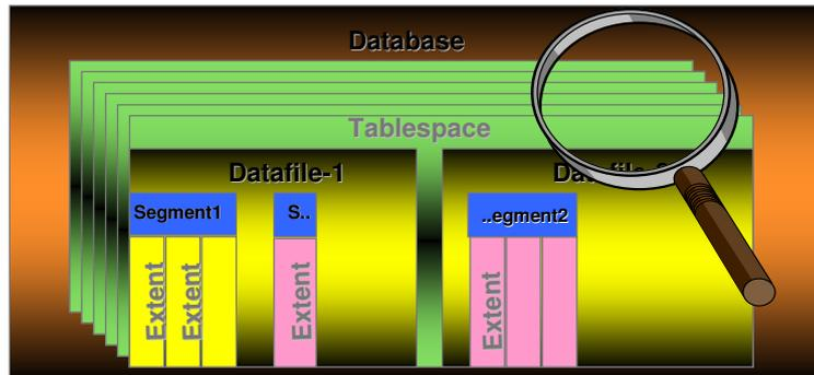
Tablespaces are nothing more than sequences of blocks and do therefore not require all the advanced features of modern file systems. In particular Oracle does not need the file system to support files of any size or to support locking or access control.
