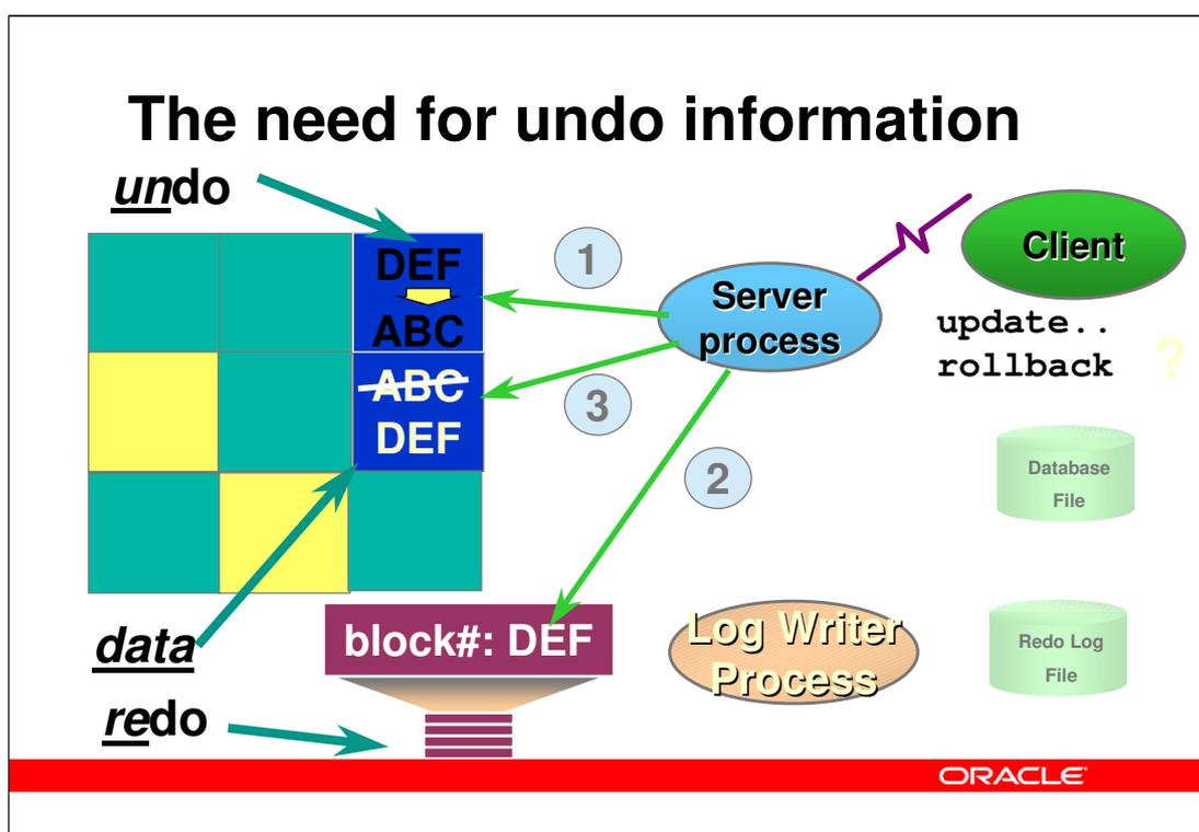
The previous slide showed the processing during normal DML operations, i.e. where the client eventually commits the operation. However, clients may want to undo the operation by performing a rollback in stead of the commit, and the simple picture does not show this. On this slide, the details of undo processing is shown.
